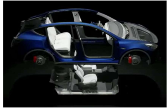
Fig. 6. Inserting the structural battery [26]
