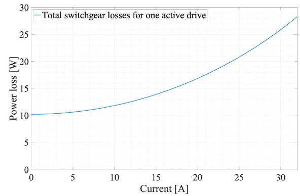
Fig. 10. Total losses of switching and protection components for one active drive at DC-TN grid
