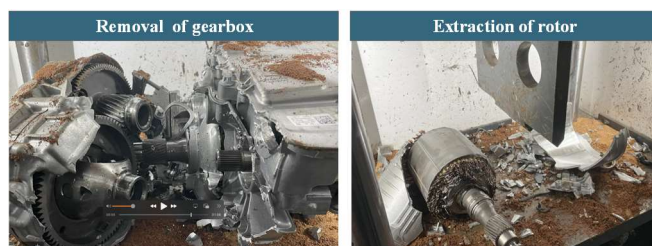
Fig. 9: Destructive rotor extraction based on hydraulic tool
