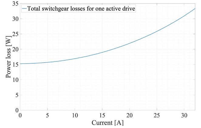
Fig. 14. Total losses of switching and protection components for one active drive at DC-IT grid
