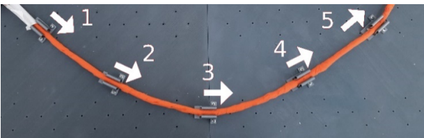
Fig. 8. 60cm cable after being automatically fed into 5 one-piece clips.
