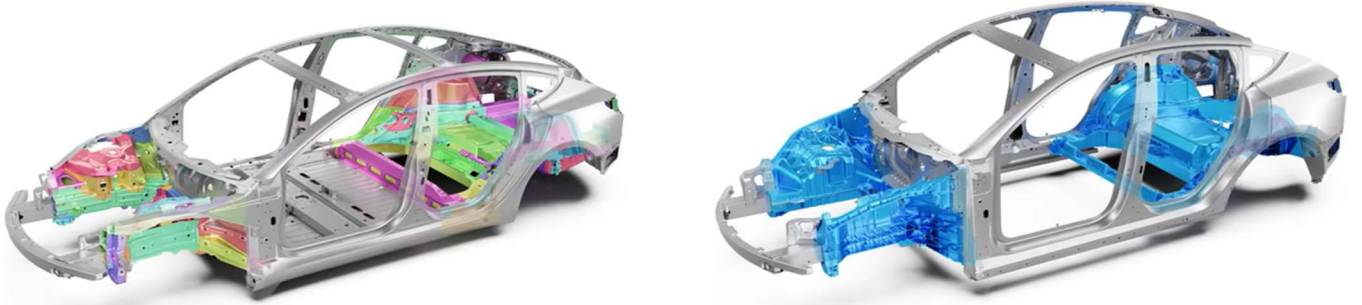
Fig. 5. Comparison between Model 3 with 171 and Model Y only 2 parts in front and rear body [24]
