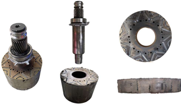
Fig. 12: Dismantling of rotor structure with hydraulic press
