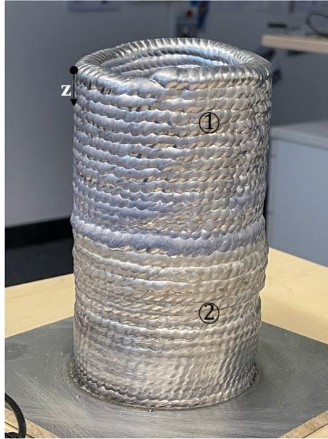
Figure 64: Additively manufactured tube consisting of multiple materials.
