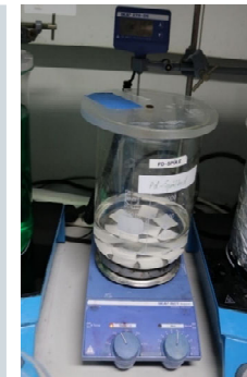
Fig. 04: Bodies debinded in Aceton bath at FAPS
