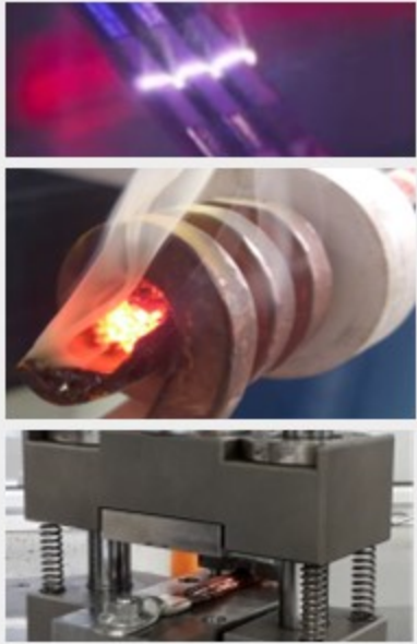
Insulation stripping and crimping
